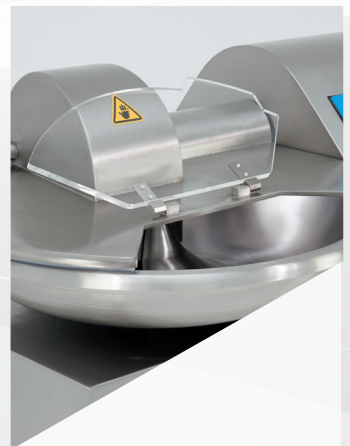
Cutter hood with transparent noise protective lid
